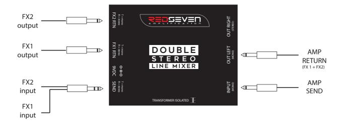
**Example 3 -** Two mono effects with two guitar amplifiers (or stereo power amplifier).
