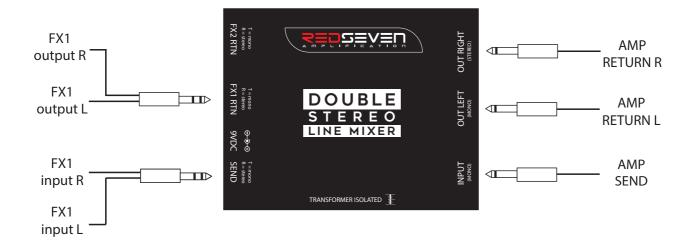
**Example 5 -** Two stereo effects with two guitar amplifiers (or stereo power amplifier).
