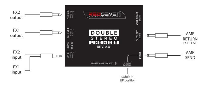
**Example 3 -** Two mono effects with two guitar amplifiers (or stereo power amplifier) – hard panned.
