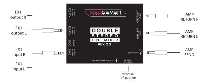
**Example 5 -** Two stereo effects with two guitar amplifiers (or stereo power amplifier). Stereo input as well.
