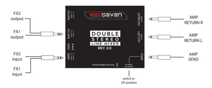
**Example 4 -** One stereo effect with two guitar amplifiers (or stereo power amplifier).
